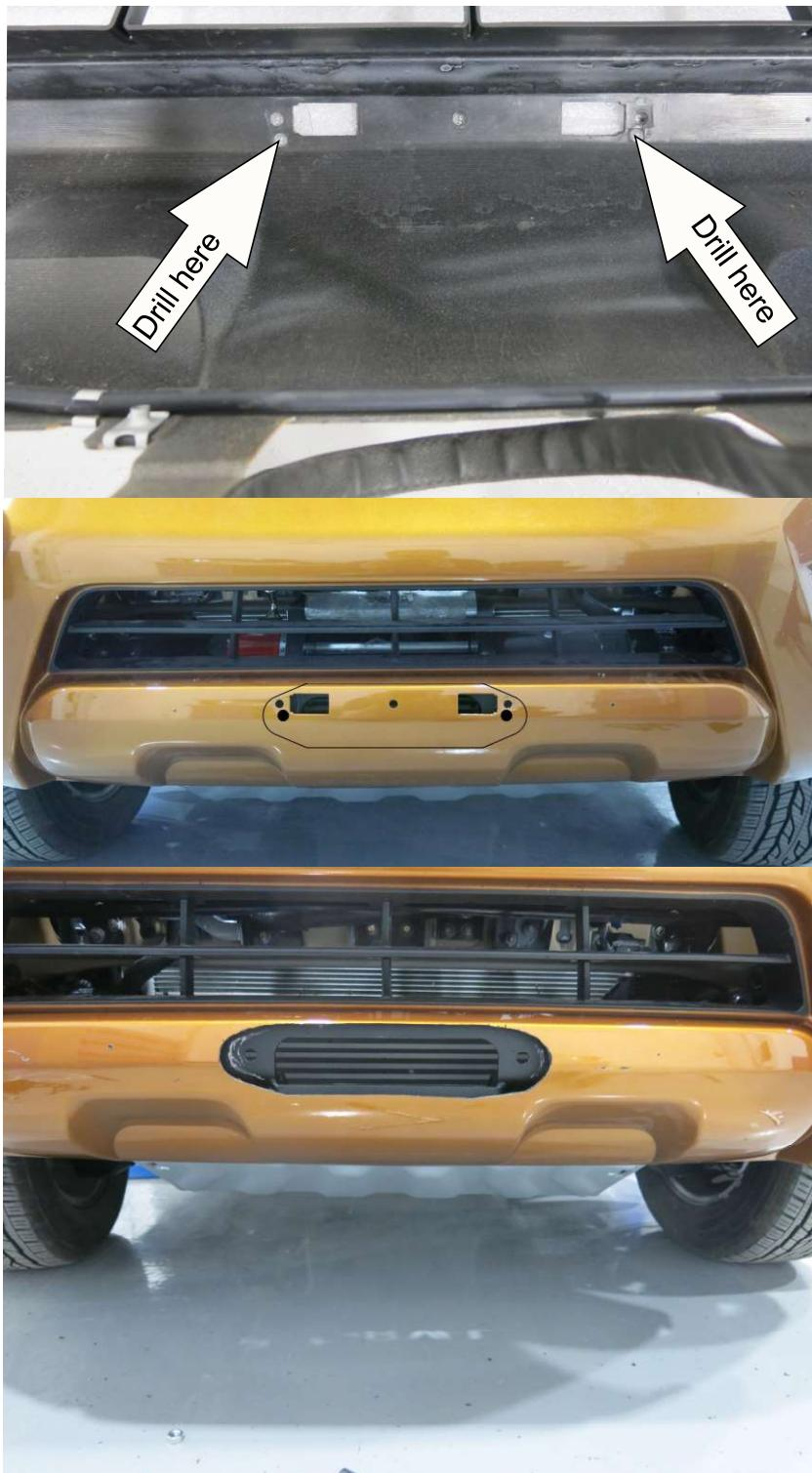
26. Temporarily install standard bumper for pad eye hole spacing. Mark the hole for pad eye fasteners on the inside of the bumper along the winch bracket.
