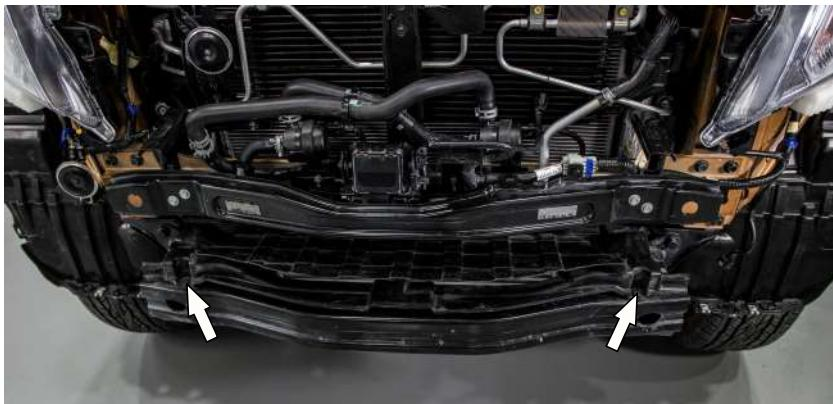
18. Remove the air intake clips.
