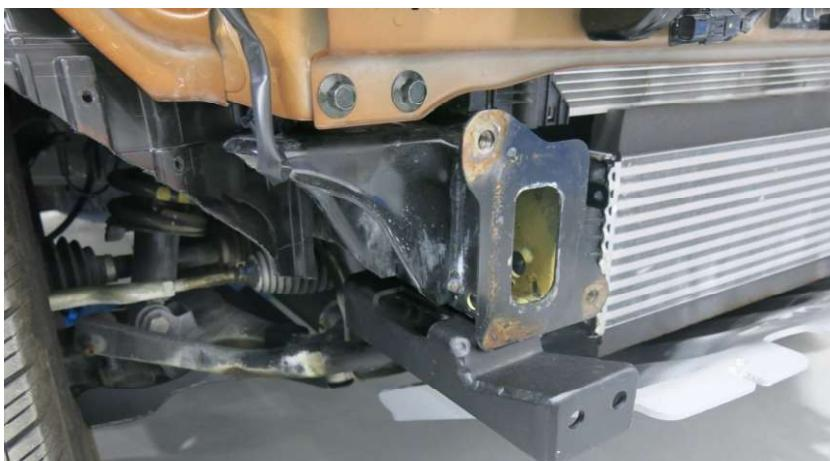
23. Install right frame booster (pos. 3) onto the vehicle frame, secure with standard bolts with installation of standard towing eye. Do not tighten screw joints.
