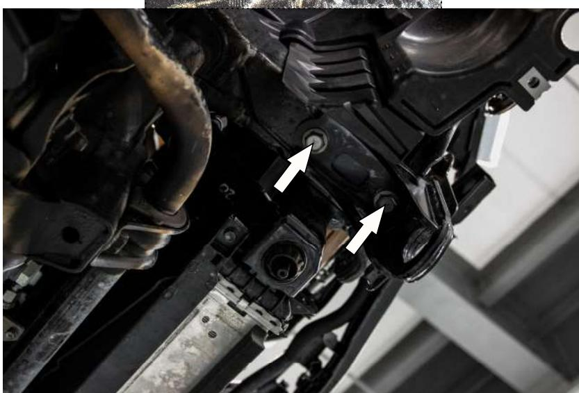
20. Unscrew 2 tension bolts of standard towing eye. Dismantle the towing eye.
