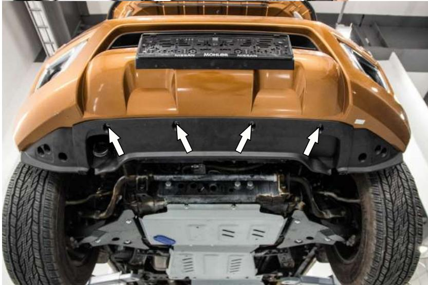
9. Unscrew 4 tension bolts of the bumper skirt center. Remove the bumper skirt center.
